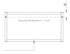
Once hooked firmly, secure the structure to the wall with a normal screw through the hole (Type A or B) made in the universal profile
