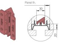
Note: The fixing of these brackets is on the front edge thereby eliminating the need of internal screwing and providing cleaner aesthetics inside the cabinet.
