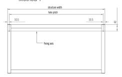
Drill holes of Ø 4.5 mm on the vertical profile in the position demonstrated in the drawing. The type of hole to be drilled depends on the fixing screw - Type A or Type B (details on the next page).
