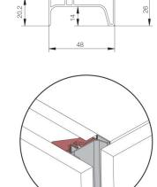
Note: These vertical profiles snap onto special brackets, which ensure firm coupling between the two components
