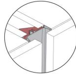
Note: These vertical profiles snap onto special brackets, which ensure firm coupling between the two components
