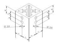
K = 8.7 mm with an end cap at the top K = 9.7 mm without an end cap at the top
